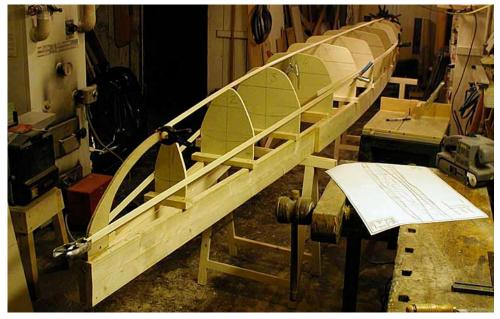
From the start I have focused on simplifying the strip building methods as far as possible, to provide the best conditions for the amateur builder to produce a functional and beautiful boat in reasonable amount of time, but also to minimize building time for the professional boat builder – a first time builder usually takes between 100 and 150 hours on a kayak project and the pro needs less than 40 hours. This Norwegian builder spent some time on the internet before choosing my Nomad:
